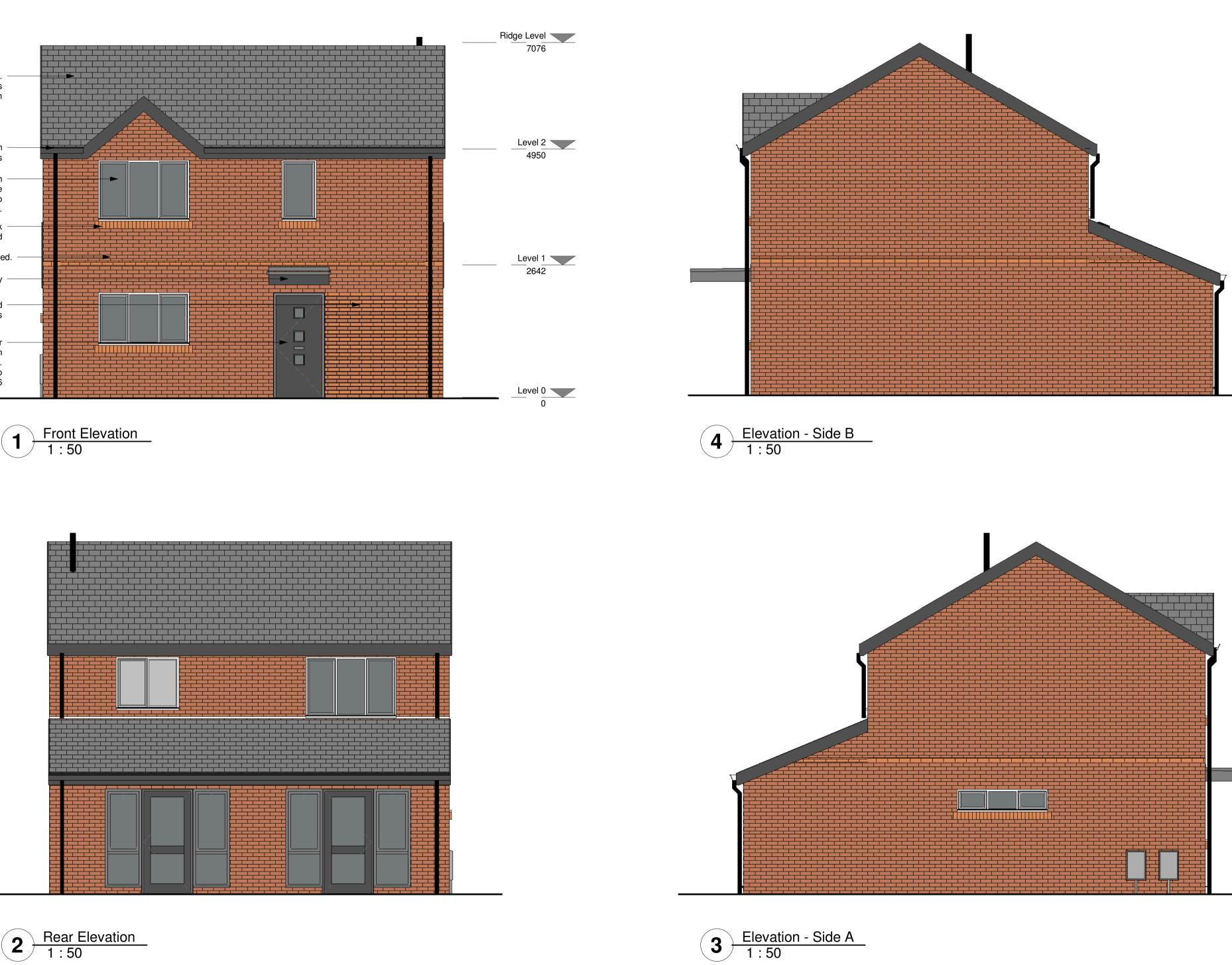
Russel Grampian Slate Grey. -concrete single lap roof tiles and system
